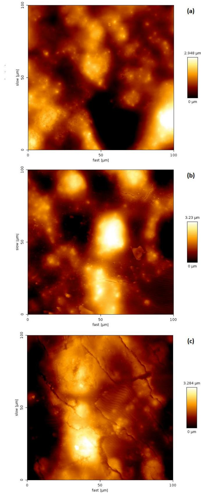
**Figure 2.** Atomic force microscopy (AFM) height map images of 100x100µm areas of Bank of Scotland £5 (a) mint and (b,c) lightly handled banknotes, showing development of surface cracking.
