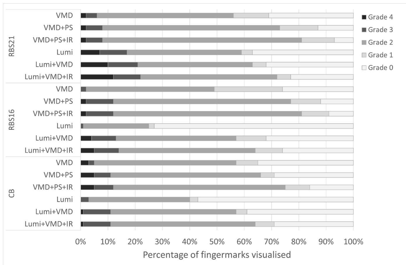
**Figure 17.** Breakdown of fingermark grades by bank and issue date, showing performance of technique or sequence of techniques, on circulated £10 notes.
