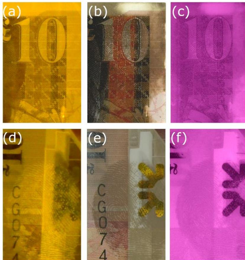
**Figure 18.** Fingermarks on RBS £10 banknotes developed with Lumicyano (a,d) showing an identifiable mark (d) and an area of note with no indication of a mark following the Lumicyano process (a). The equivalent areas are shown in (b,e) respectively with a subsequent VMD process, the Lumi+VMD sequence showing ridge detail in both cases. IR imaging (c,f) in this instance does not add substantial benefit.
