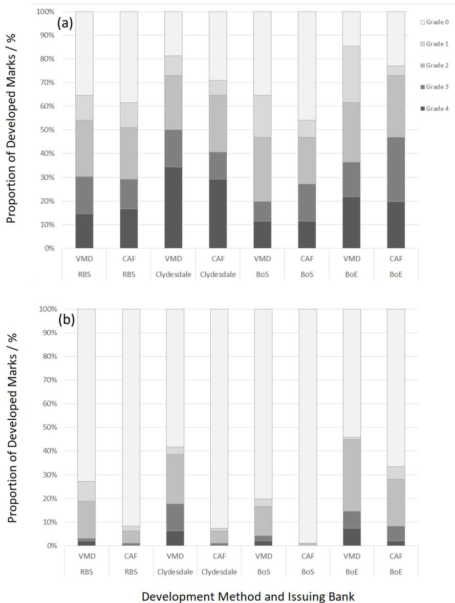
**Figure 7.** CAST grades of fingermarks developed on £5 banknotes on (a) mint and (b) handled notes with VMD and CAF development across all banks.
