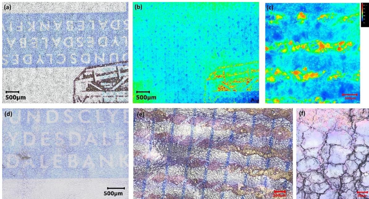
**Figure 1.** Surface structures of heavily handled Clydesdale Bank £5 note studied by LCSM (a-c) mint and (d-f) handled note. (a) image and (b) corresponding height map of opaque area, with intaglio features in bottom right. (c) intaglio shading from portraiture. Height map scale is  $25\mu\text{m}$ . Degradation with handling in (d) and (f) opaque polymer, and (e) showing removal of intaglio features, with degradation of polymer.
