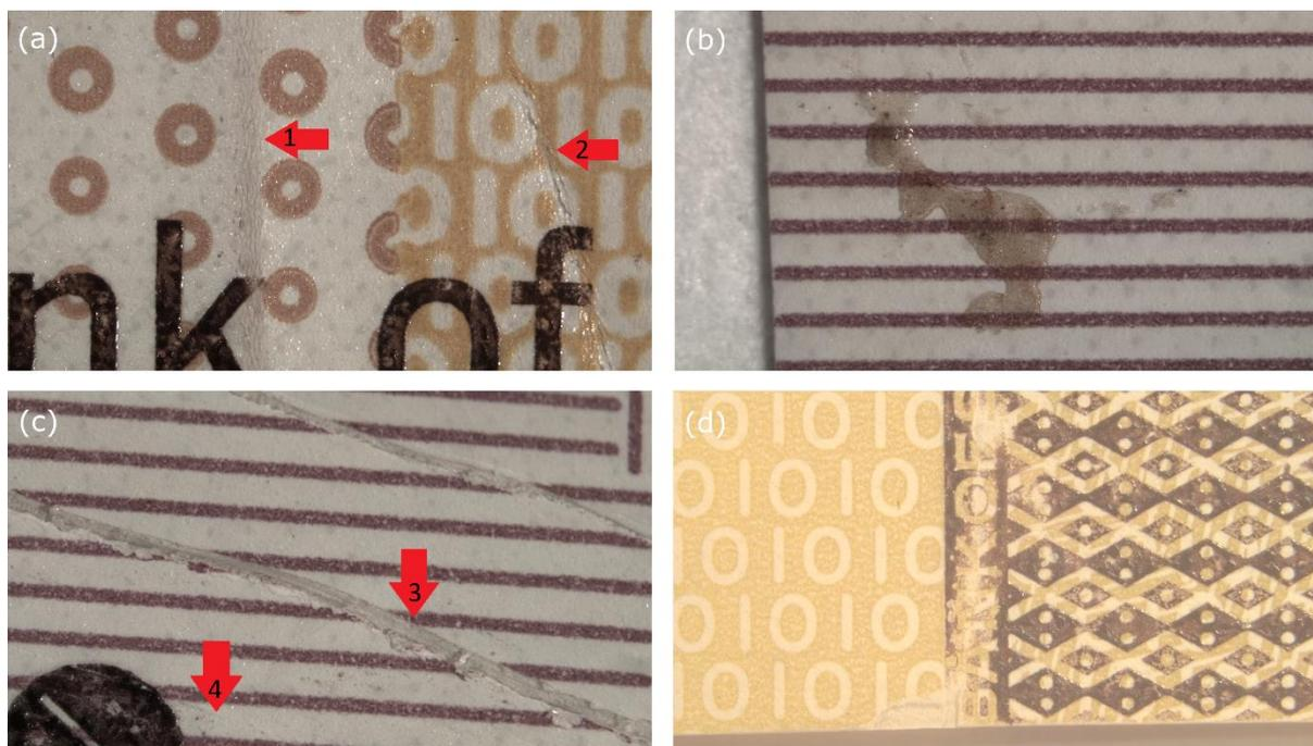
**Figure 8.** Example light microscopy images of circulated Bank of Scotland £10 banknotes, showing different types of damage. (a) and (c) show linear damage, arrows indicate multiple features within images, 1) light cracking 2) deep cracking 3) heavy scratches 4) light scratches. b) Contamination and d) pattern damage are also shown. Approximate magnifications a) 16x, b,c) 20x, d) 12x.
