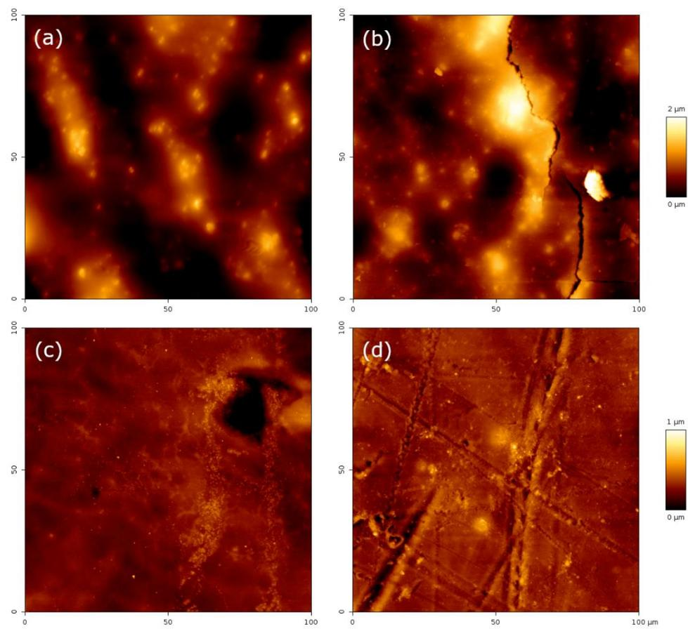
**Figure 12.** Atomic force microscopy height images of 100x100 μm areas of (a,c) mint and (b,d) circulated Bank of Scotland £10 notes, (a,b) Spark region with height colour scale of 2 μm (c,d) transparent polymer region with height colour scale of 1 μm.
