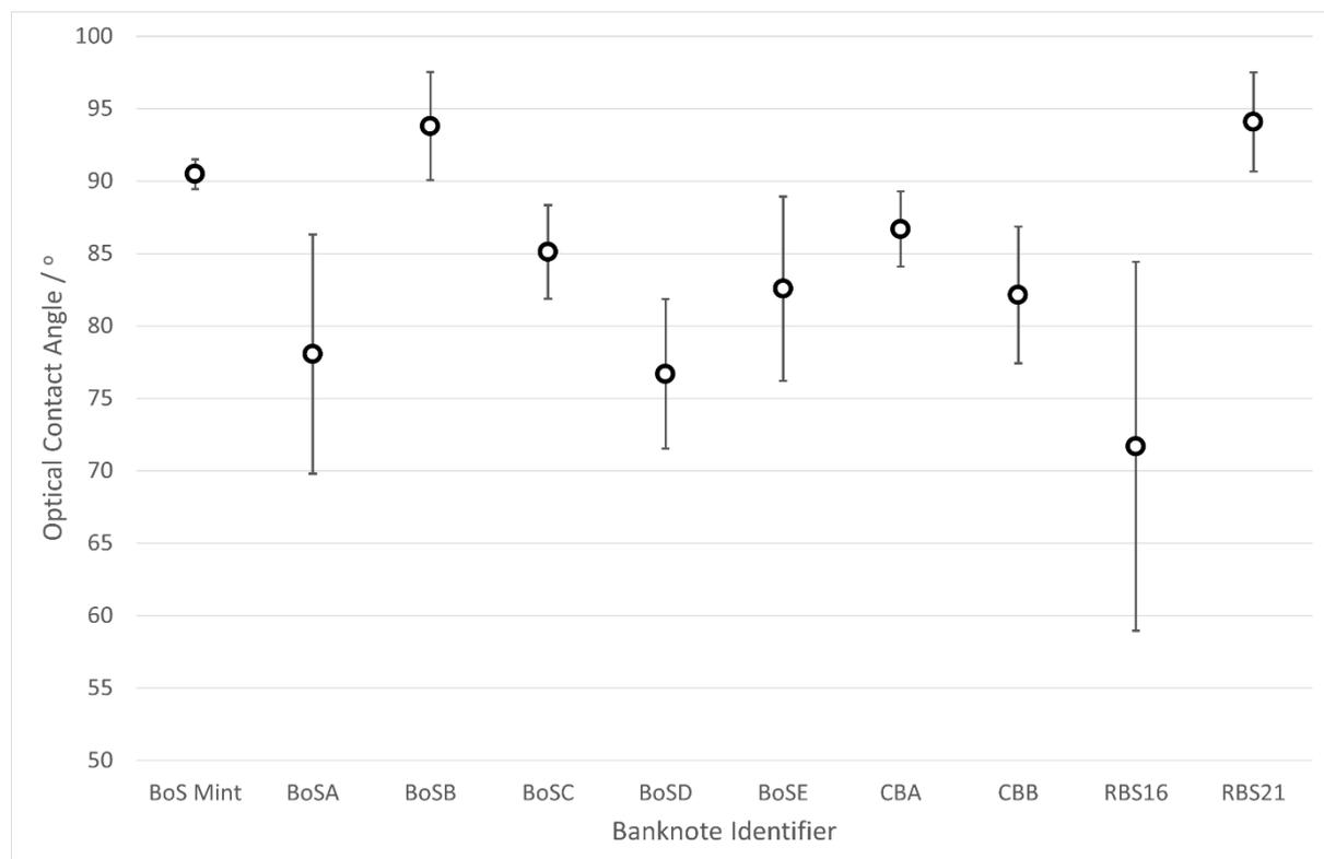
**Figure 13.** Wettability of the banknote surface from optical contact angle measurements of opaque polymer region of individual £10 banknotes.
