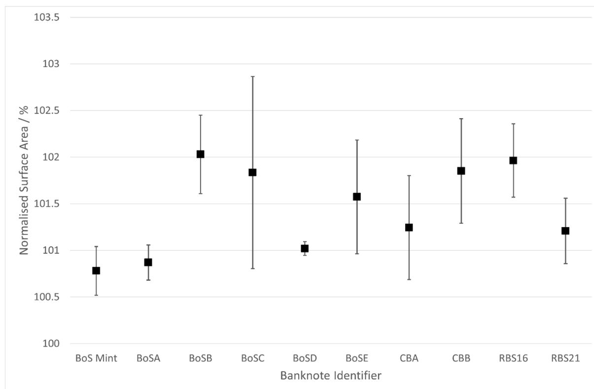
**Figure 10.** Surface roughness factor,  $R_{SA}$  of the banknote surface from atomic force microscopy measurements of opaque polymer region of individual £10 banknotes.
