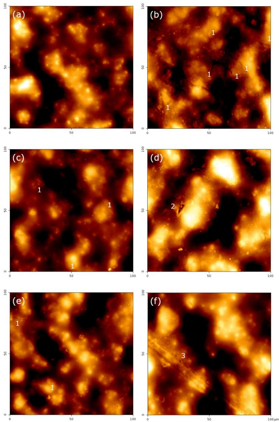
**Figure 11.** Atomic force microscopy height images of 100x100  $\mu\text{m}$  areas of £10 banknotes, (a) mint and (c,e,f) circulated Bank of Scotland notes, circulated (b) Royal Bank of Scotland 2016 issue and (d) Clydesdale Bank issue. With (1) microcracking (2) micro scale holes and (3) macro scratches. Height colour scale of 2  $\mu\text{m}$  on all images.
